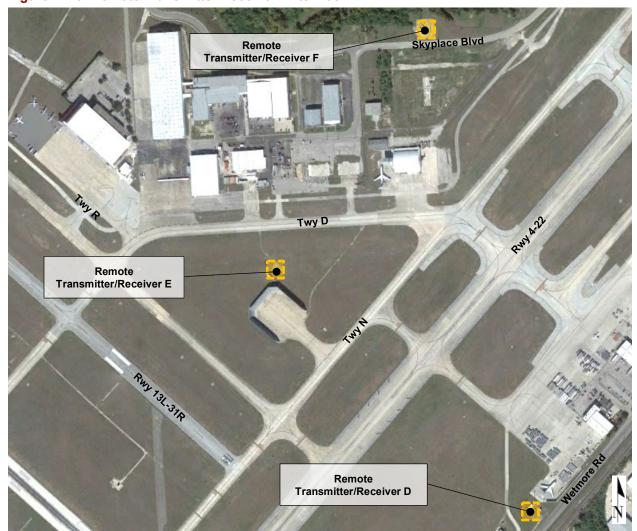
Figure 2.7-9: Remote Transmitter/Receiver Antennas
