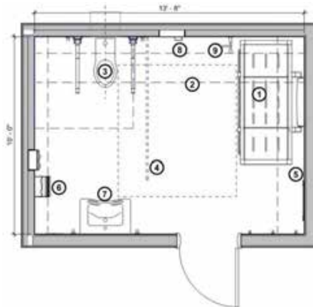
Figure 40: Typical Companion Care Restroom Layout
