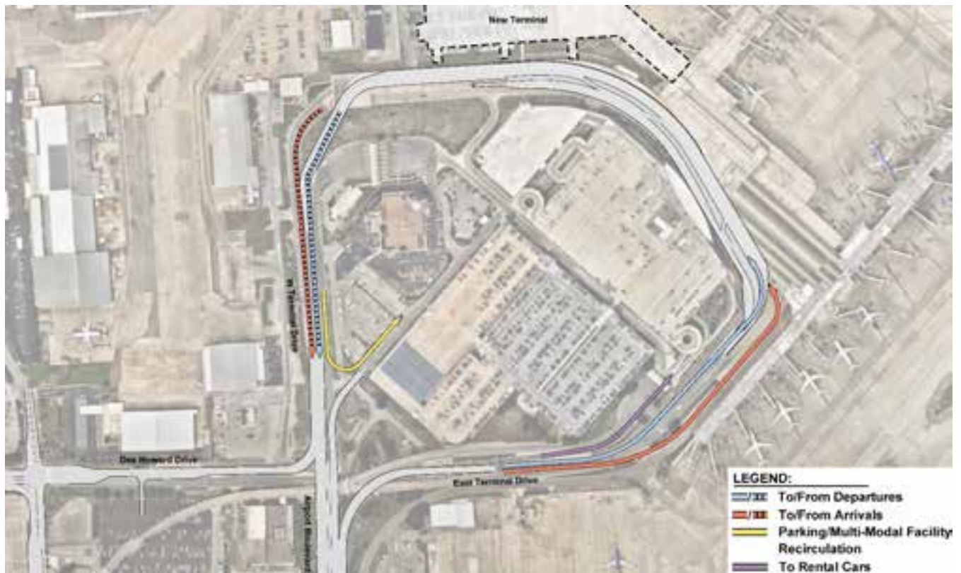
Figure 5: Functional Curbside Circulation
