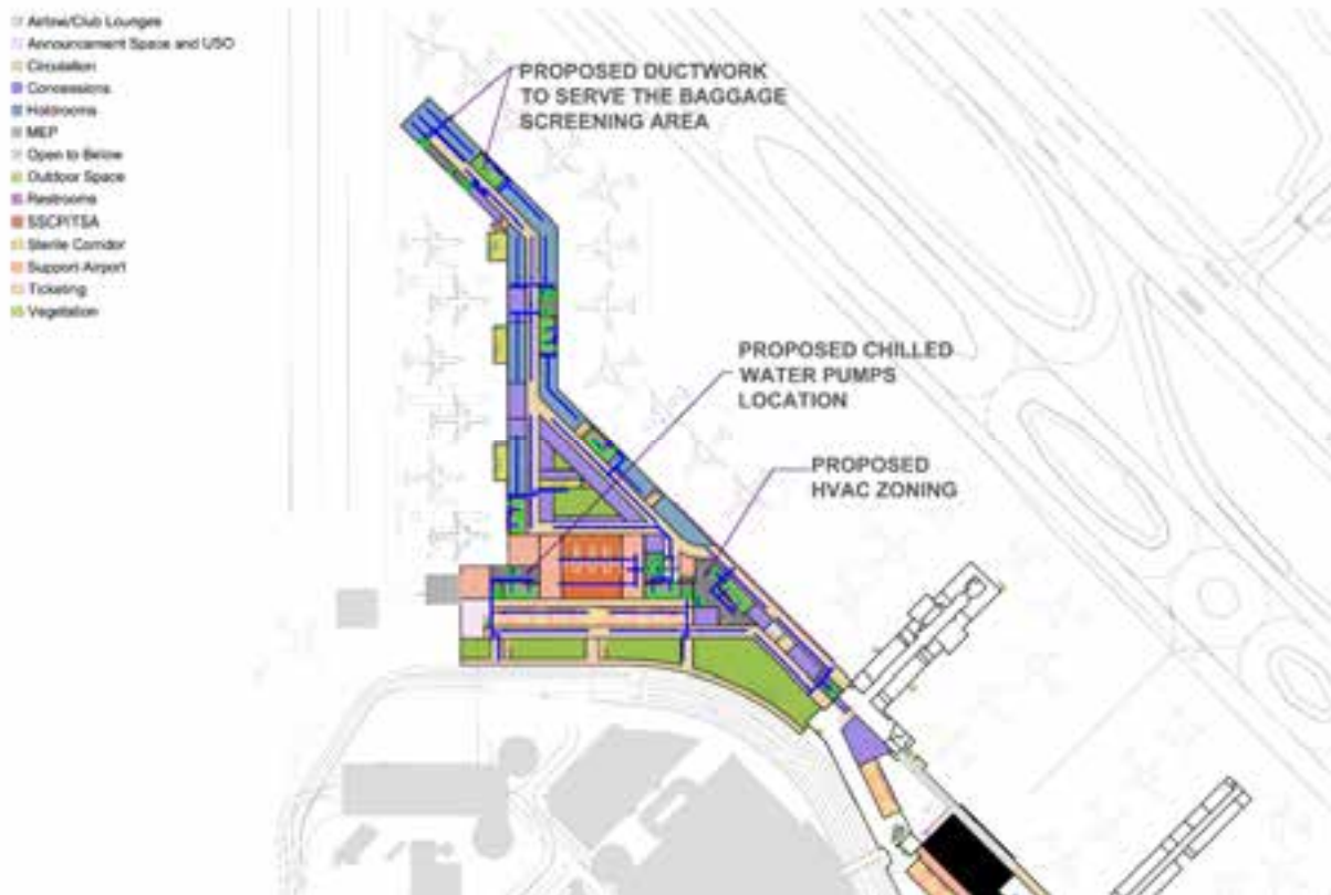
Figure 73: Departure Level Proposed HVAC Units
