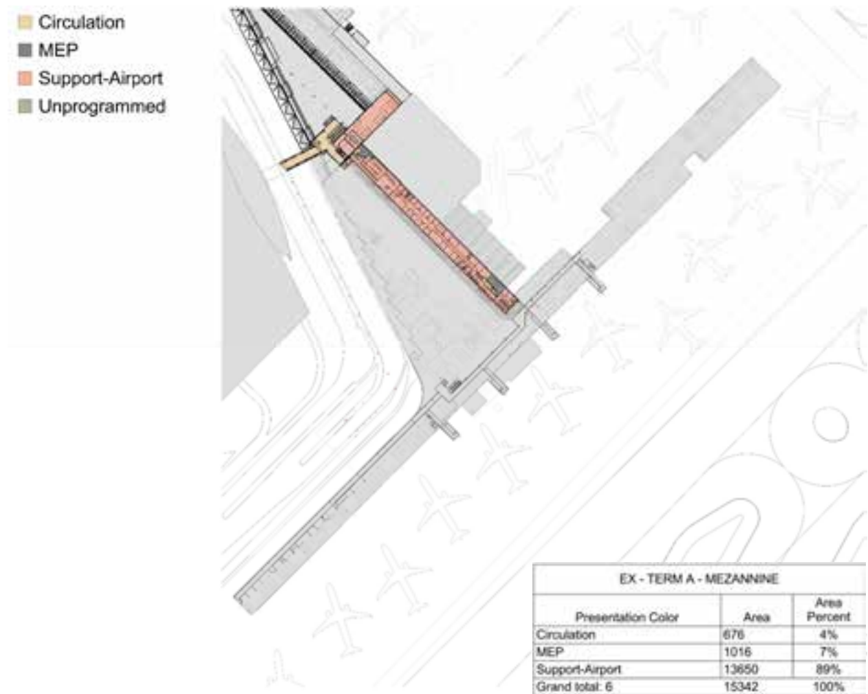
Figure 14: Terminal A - Existing Mezzanine Level
