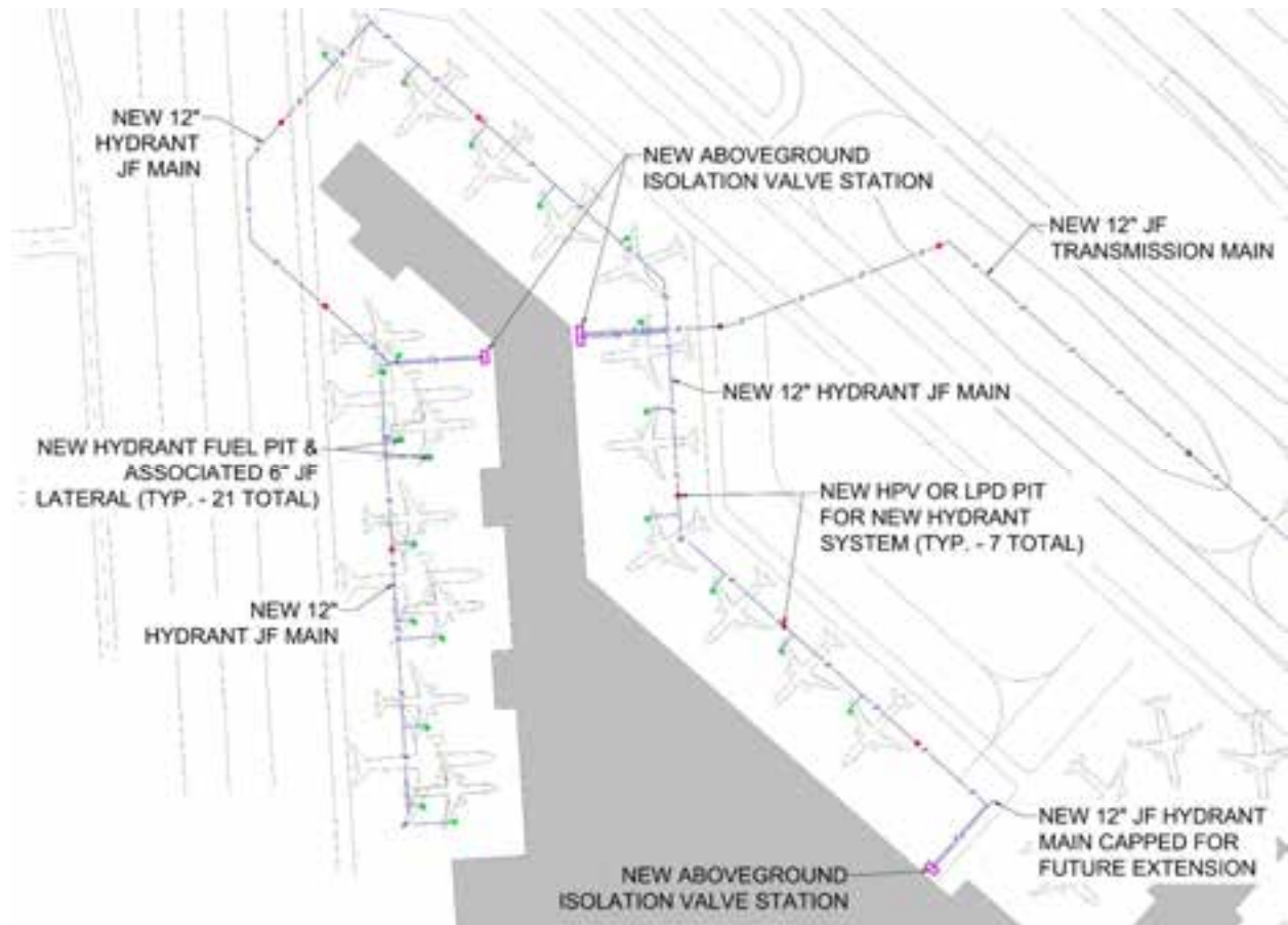
Figure 34: New Terminal Hydrant Fuel System
